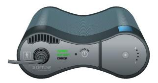
If a wall power supply is plugged into the device the device will run using the wall power supply and the "Battery" indicator will not illuminate.
