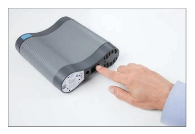
**5.** Allow about 10 seconds for the self-check to be completed. The "Power" indicator on the front panel of the device will illuminate green.
