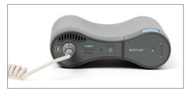
If a charged battery is installed and there is no wall power supply plugged in, the "Battery" indicator will also illuminate green.
